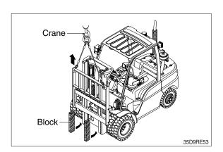
② While supporting lift chains, remove the split pin and nuts from the anchor bolt. Slide out chain anchor bolt from the chain anchors of stationary upright.
