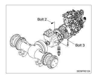
③ Using a moving truck slowly pull out transmission assembly to the front.
